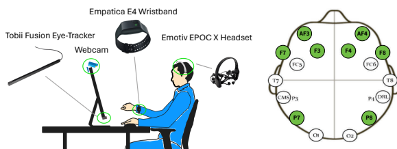
Figure 3: Experiment setup (left), and the EEG electrode locations (right). The filled circles indicate the electrodes used to compute the indexes.
