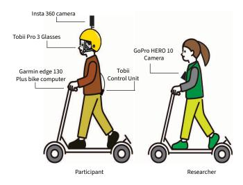
Figure 1: Participant equipped with Insta 360 camera, Tobii Pro 3 Glasses, Garmin edge 130 Plus bike computer and a following rider equipped with GoPro HERO 10 Camera.
